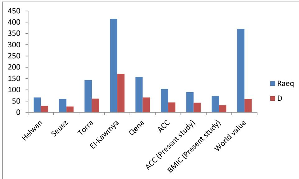
Fig.8: Comparison of  $R_{aeq}$  and absorbed dose rate (D) for Portland cement samples from ACC & BMIC with those from Egyptian cement factories [16].
