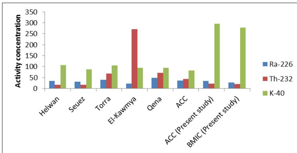
Fig. 5: Comparison of average activity concentration (Bq/Kg) of Portland cement samples from ACC & BMIC with Egyptian cement factories <sup>[16]</sup>.
