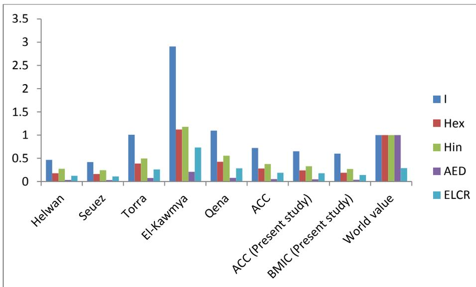
**Fig.7:** Comparison of some hazards indices for Portland cement samples from ACC & BMIC with those from Egyptian cement factories<sup>[16]</sup>.
