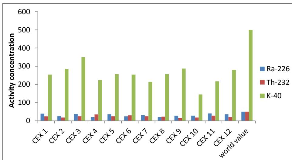
**Fig.3:** Comparison between activity concentration of  $^{226}\text{Ra}$ ,  $^{232}\text{Th}$  and  $^{40}\text{K}$  from ACC cement product with world value.
