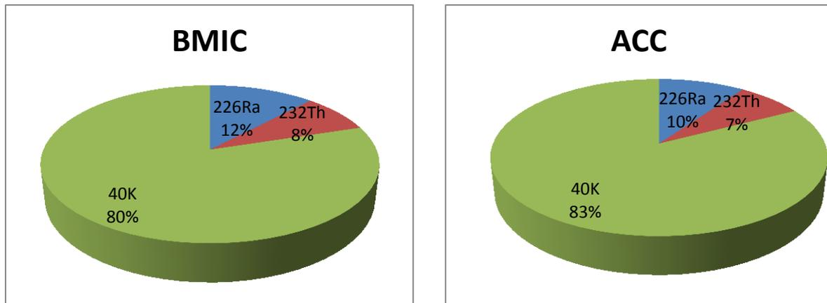
**Fig.2:** Percentage contribution of the three naturally occurring radionuclides in the cement product from ACC & BMIC.
