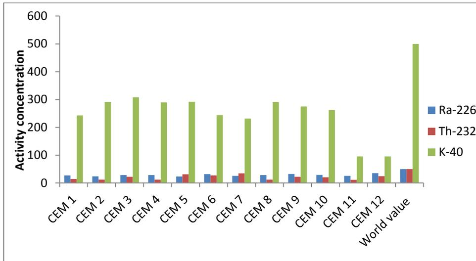
Fig.4: Comparison between activity concentration of  $^{226}\text{Ra}$ ,  $^{232}\text{Th}$  and  $^{40}\text{K}$  from BMIC cement product with world value.
