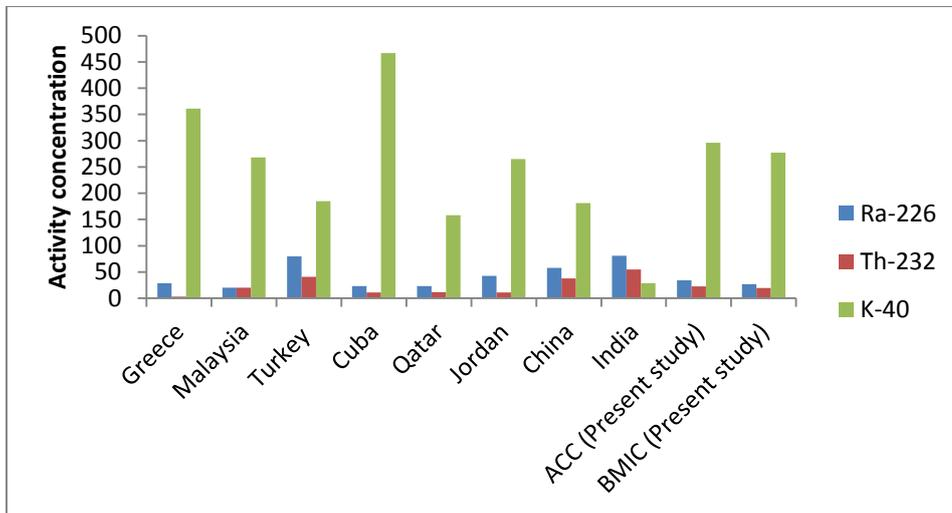
**Fig. 6:** Comparison of average activity concentration (Bq/Kg) of Portland cement samples from ACC & BMIC with world cement factories<sup>[16]</sup>.
