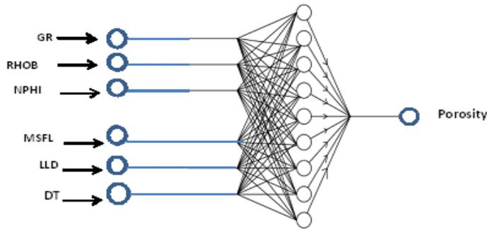
Figure 4: schematic of developed ANN model for porosity
