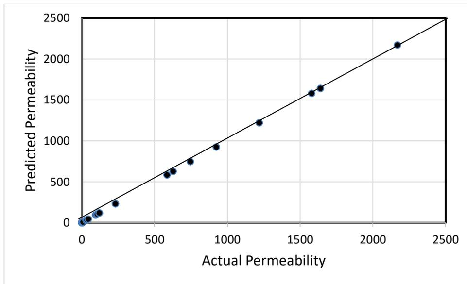
Figure 10: Crossplot of estimated permeability from ANN model and core permeability data. (Training data)
