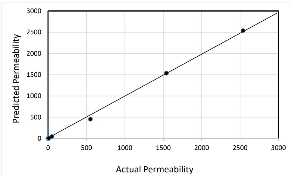
Figure 12: Crossplot of estimated permeability from ANN model and core permeability data. (Validation data)
