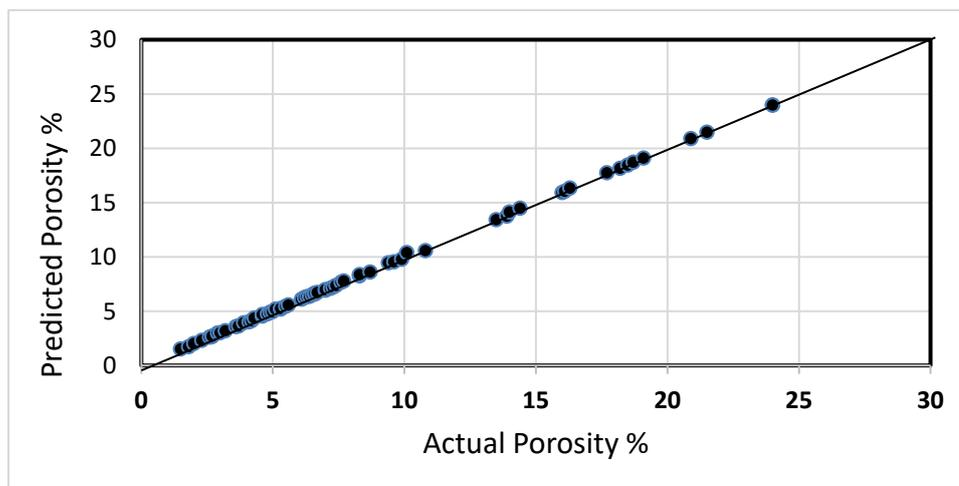
Figure 6: Cross plot of predicted porosityfrom ANN model and core porosity data (training data)
